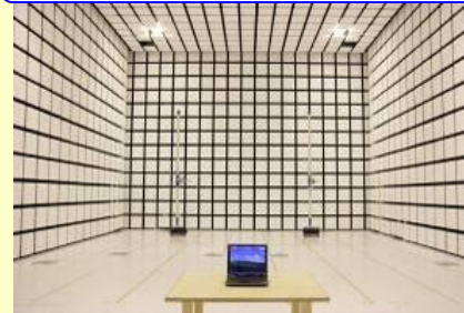
(10m法電波暗室)
