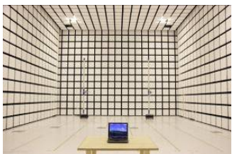
(10m法電波暗室)
