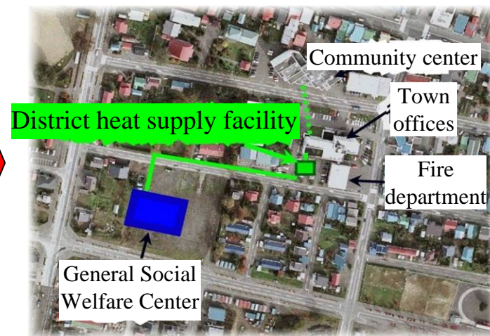
District heat supply powered by a wood boiler
